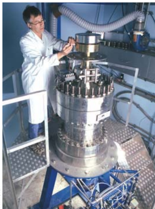
The HETIQ (HElium Tightness Qualification) test rig, set up at the CEA Cadarache Center, developed to carry out testing, and qualification of all gastight sealing devices likely to be encountered in a GFR, under representative conditions.
