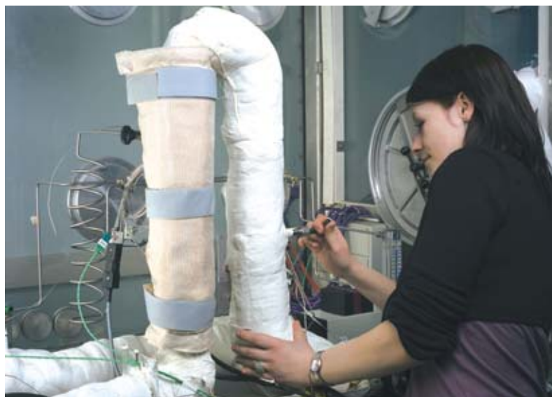
Optimizing the helium purification process on the CIGNE chemical reactor. Helium quality is of paramount importance, since the impurities in this coolant gas determine its corrosive potential with respect to structural materials.
